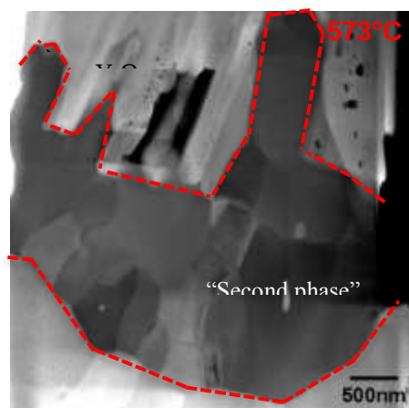
Figure 43. a) HAADF image of the Y_2O_3 /second phase/V-4Cr-4Ti interface exposed to 573 °C. b) EELS spectrums indicating no Li present.
