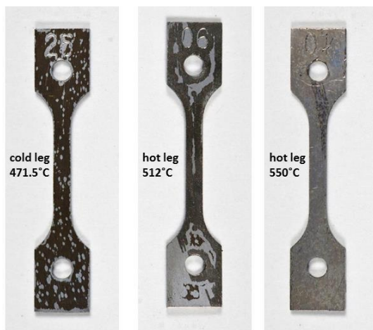
Figure 31. Appearance of loop specimens following exposure at the indicated temperatures. Note that as the temperature increases, less of the surface is covered by the relatively dark aluminum-rich film.
