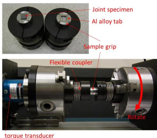
Figure 33. Torsional shear test apparatus.
