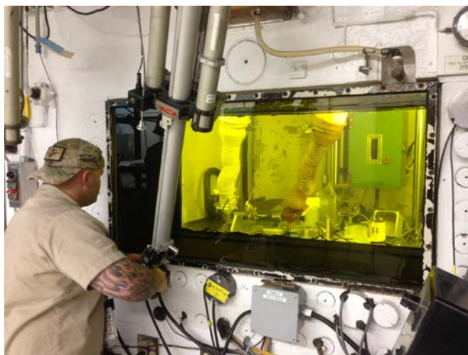
Figure 91. HFIR irradiation capsule disassembly by remote manipulation in the IMET Hot Cells in ORNL Building 3025E.
