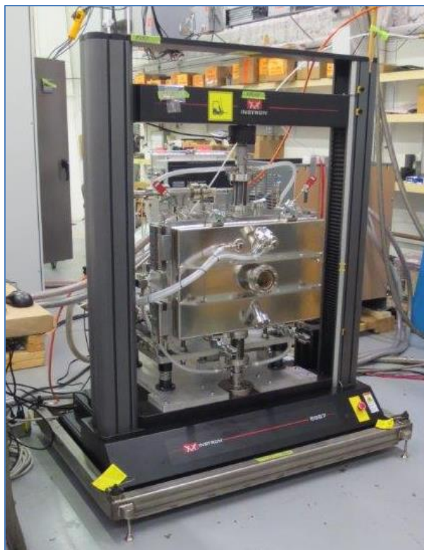
Figure 64. Front and Rear Views of Oxy-Gon Custom Vacuum Chamber on an Instron Load Frame Ready for NRTL Inspection and Factory Acceptance Test in October 2016.
