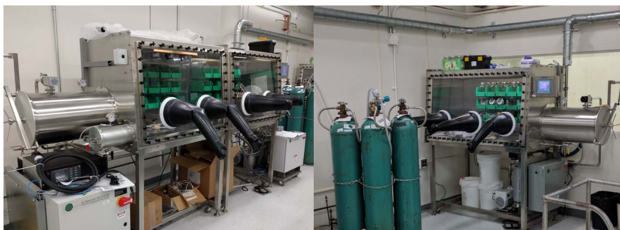
Figure 19. New glove boxes for handling liquid metals in an inert (Ar) environment. Left: large glove box with O 2 , H 2 O and N 2 control. Right: smaller glove box for cutting Pb-Li.
