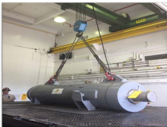
Figure 66. Shipping cask that will be used for RB-19J capsule (a) Handling of the loop cask container and (b) loading of the loop cask container.
