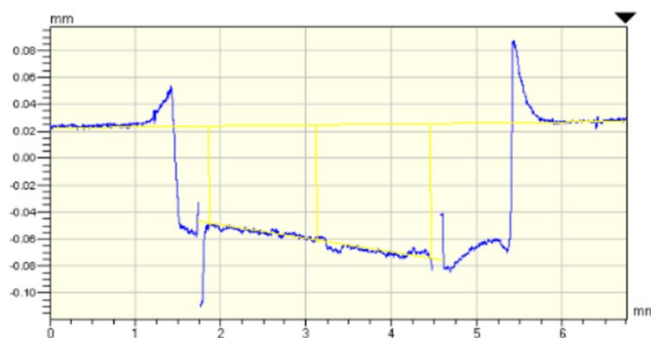
Figure 61. Example of sputtered crater depth profile. The slope at the bottom of the crater was because the original sample was not mounted flat in the mount.
