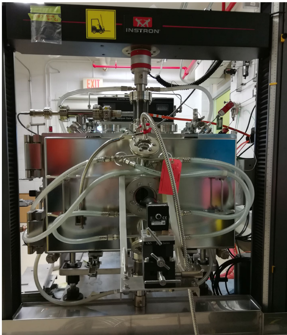
Figure 54. Front view of the high temperature vacuum test frame ready for installation in the IMET hot cells of ORNL Building 3025E.
