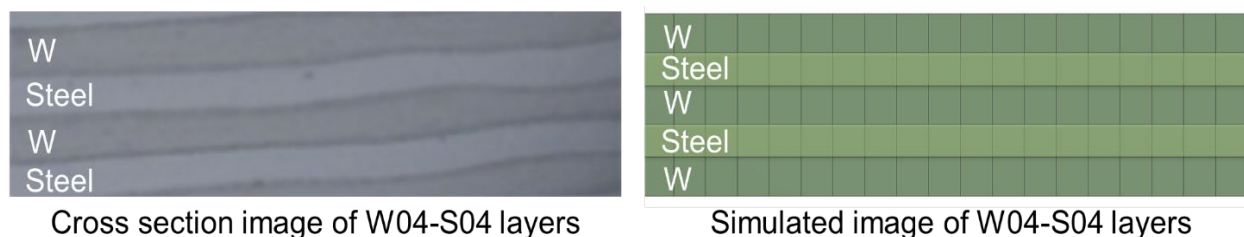
Figure 58. Cross section of experimental tungsten-steel laminate (left). Simulated tungsten-steel laminate layers with 57 \mu\text{m} individual layer thickness (right).
