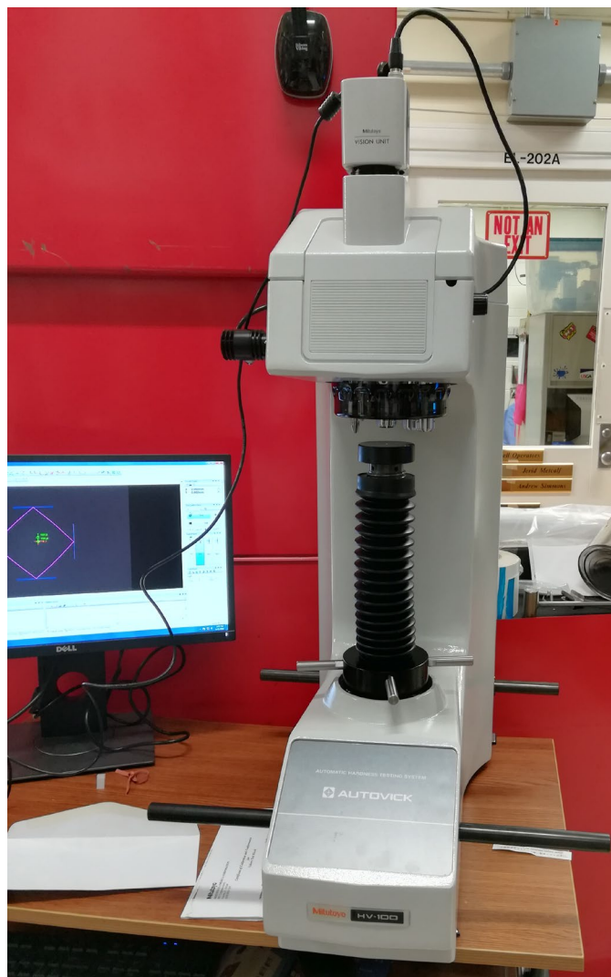
Figure 55. New Mitutoyo HV-120B Vickers hardness tester for installation in the Building 3025E hot cells.
