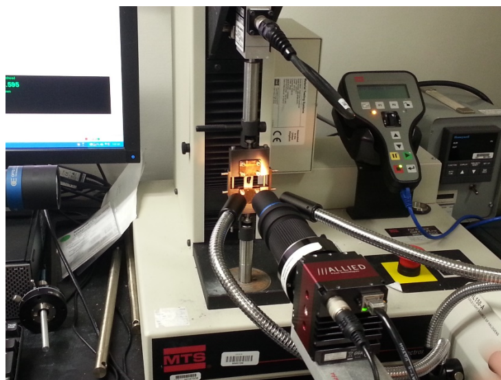
Figure 71. Fiber fixture installed in the tensile frame with the camera for digital image correlation immediately in front of the sample.
