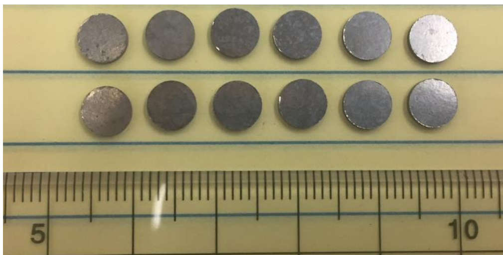
Figure 25. Appearance of W-SiC joint specimens.
