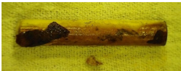
Figure 100. Irradiation capsule F8B1. Dark brown markings believed to be resin residue from fiber tube disintegration.
