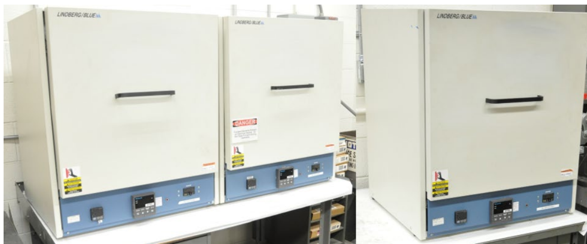
Figure 86. Lindberg/Blue M box furnaces.
