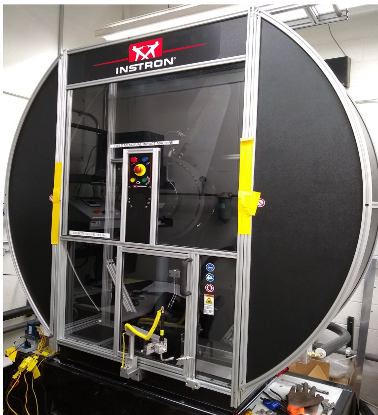
Figure 89. Instron Charpy impact frame with in-situ heating/cooling stage.
