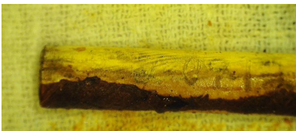
Figure 101. Irradiation capsule F8B2. Dark brown at bottom of tube believed to be resin residue from fiber tube disintegration.
