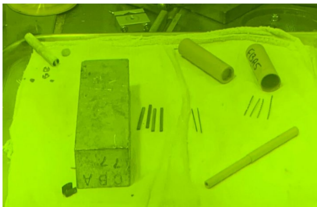
Figure 99. Image of disassembled F13A5 components. Four M3PCCVN bars are pictured center with SiC TMs to the right of them.
