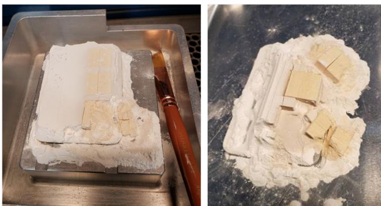
**Figure 79.** Photograph showing the results from the first attempt of binder jet print at ORNL. The resultant material was not adequately consolidated.
