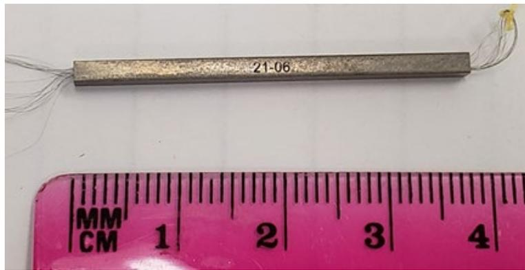
Figure 98. W fiber container with fiber specimens prior to fiber ends trimmed.
