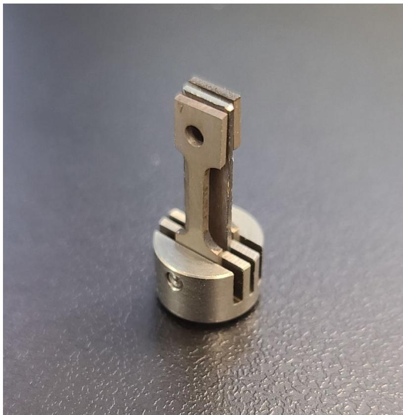
**Figure 105. Frontier Task 3 molten Sn rabbit capsule specimen region assembly.**
