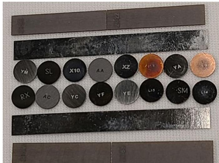
Figure 102. W and W/Cu 6 mm diameter disc specimens.
