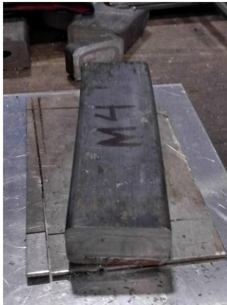
**Figure 25. Cross-section of the extruded M4 bar showing the ODS section enclosed in the steel can.**
