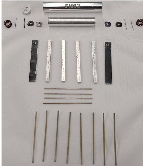
**Figure 107. FH62 low dose bend bar capsule components during assembly.**
