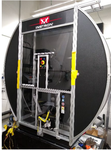
Figure 8. Instron Charpy impact frame equipped with an MPM in-situ heating/cooling stage.
