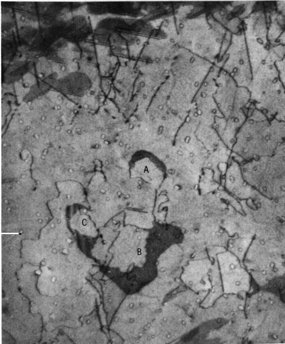
Fig. 14. Micrograph showing three Frank interstitial loops designated by letters A, B, C in neutron-irradiated Nimonic PE16 being unfaulted by perfect dislocations. Voids are also visible.
