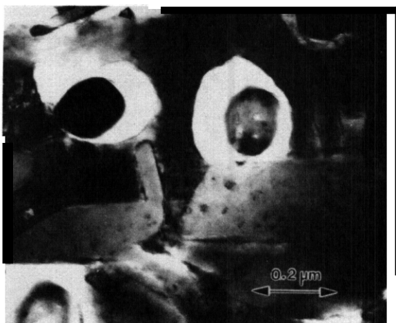
Fig. 18. SEM micrograph of the surface of an electrc-polished NMF3 specimen irradiated at 520°C to 75 dpa showing highly decomposed Y/Y grain boundaries,
