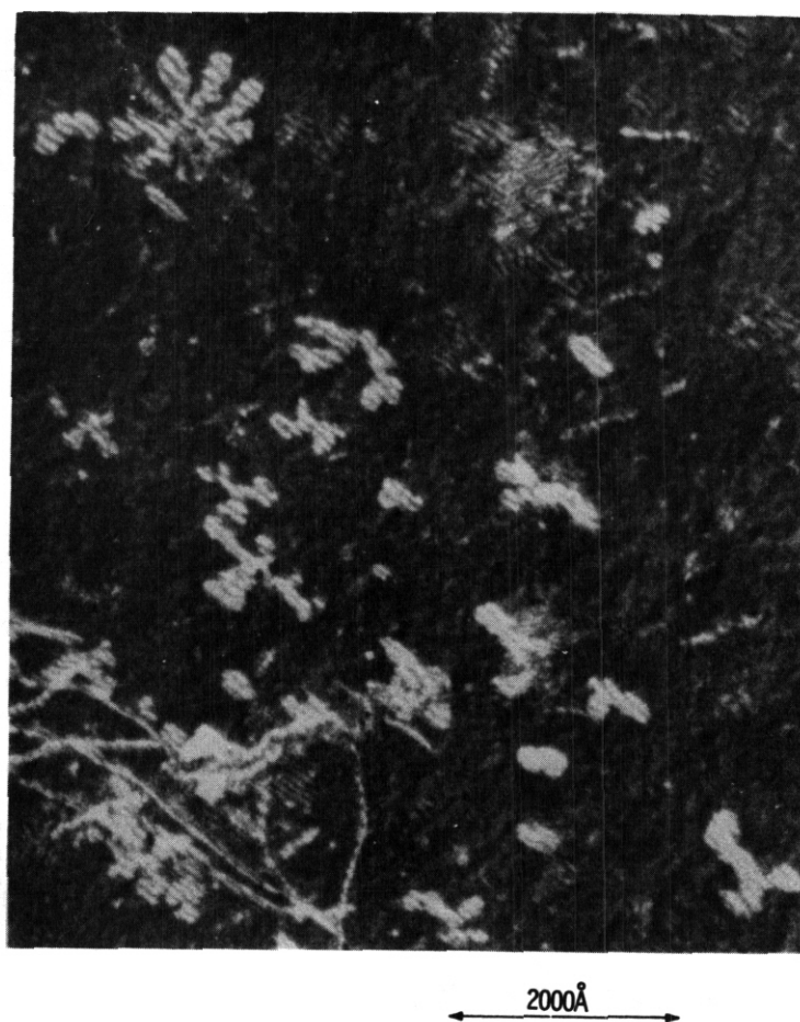
Fig. 5. Dark Field Micrograph Showing Irregular Shaped Frank Interstitial Loops observed in 304 stainless steel irradiated at 370°C to 2 dpa. 36
