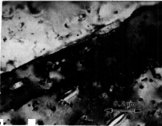
Fig. 9a. Bright field TEM image of small rectangular precipitates along a grain boundary and within the grain in cold-worked 18/18 Plus irradiated at 600°C to 60 dpa.
