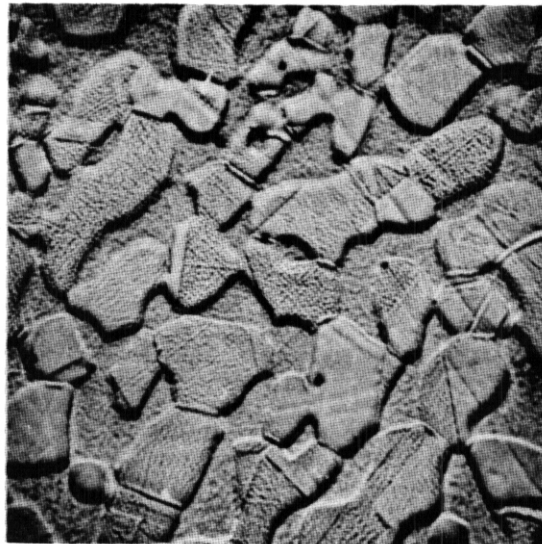
Fig. 1. Surface of a duplex alloy, Uranus 50, bombarded with 10^{17} Ni + ions/cm 2 at 625 °C. The austenite grains have swollen and risen above the adjacent low-swelling ferrite grains. No lateral expansion of the austenite grains has occurred, reflecting the unidirectional nature of the swelling. 22
