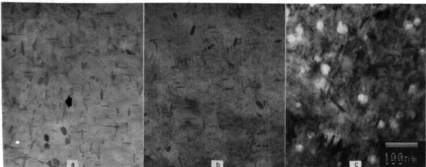
Fig. 4. Comparison of precipitate and void structures as a function of V content for specimens irradiated at 420°C to 115 dpa a) 2Cr-0.5V alloy L1, b) 2Cr-1V alloy L2 and c) 2Cr-1.5V alloy L3. The imaging conditions used in c) do not show the precipitate particles clearly
