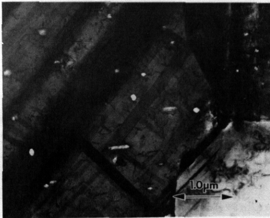
Fig. 23a. Bright field TEM image of M_{23}C_6 at grain boundaries, large voids (some elongated) and stacking faults within \gamma grains in NMF3 irradiated at 600°C to 60 dpa.
