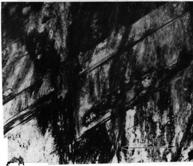
Fig. 14a. Bright field image of unirradiated cold-worked NMB showing twins and a high dislocation density.
