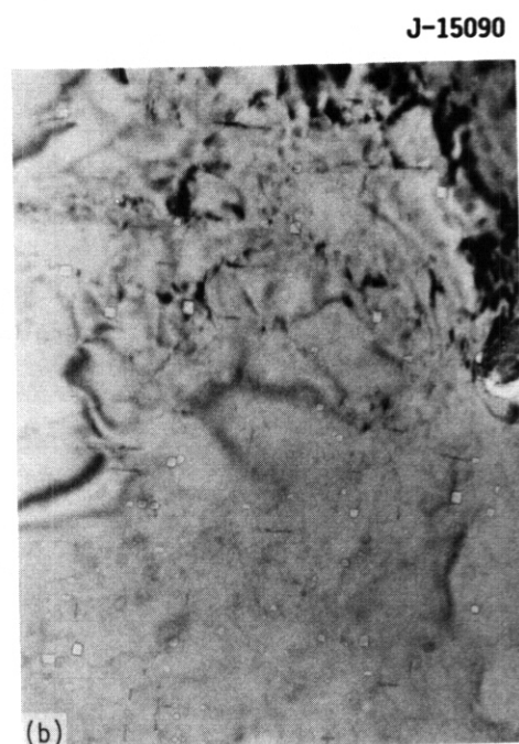
Fig. 3. Cavities in (a) annealed V-3Ti-1Si and (b) Warm-worked V-3Ti-1Si, after irradiation in FFTF at 520°C to 26 dpa. Both specimens were preimplanted with 232 appm ^3\text{He} . Note small rod-like precipitate particles.
