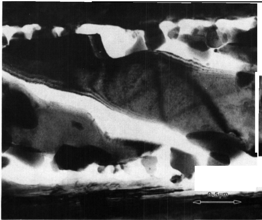
Fig. 8. Bright field TEM image at higher magnification of one of the \alpha' martensite plates in figure 7b showing M_{23}C_6 carbides at the \alpha' /austenite grain boundary and within the dislocation free \alpha' martensite
