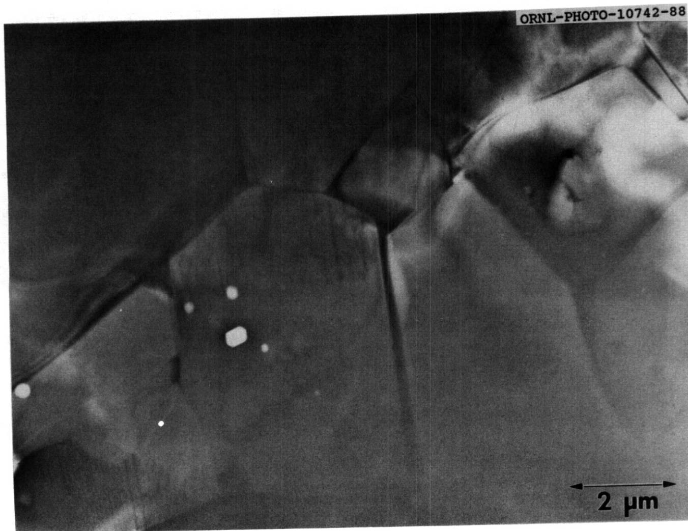
Fig. 5. General TEM microstructure of alumina calcined at 1300°C and sintered at 1700°C.
