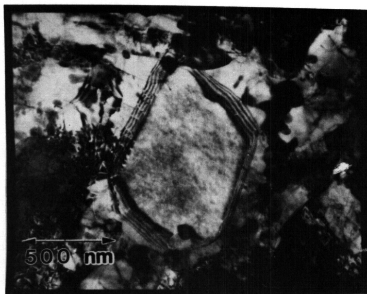
Figure 13. Recrystallized ferrite in L9 aged for 5000 hours at 520 C.
