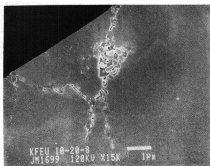
Fig. 15. SEM image of foil surface of CWA AMCR irradiated at 420°C showing preferential electropolishing at grain boundaries and regions of decomposition to \alpha -ferrite and M_{23}C_6 due to Cr depletion of the matrix by M_{23}C_6 precipitation
