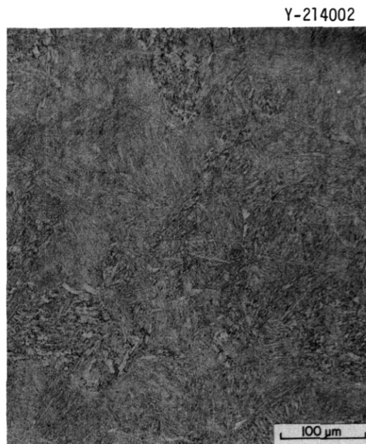
Fig. 2. Polygonal ferrite and tempered bainite microstructure of normalized-and-tempered 2 \frac{1}{4} Cr-1Mo steel.
