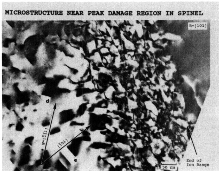
Fig. 4. Dislocation microstructure observed near the ion-implanted region of \text{MgAl}_2\text{O}_4 after irradiation with 2.4 MeV \text{Mg}^+ ions to a fluence of 1.4 \times 10^{21} ions/ \text{m}^2 at 650^\circ\text{C} . The irradiation flux was about 1.5 \times 10^{17} ions/ \text{m}^2\text{-s} . The maximum damage level and implanted ion concentration in the ion-implanted region was about 40 dpa and 5 at. %, respectively.
