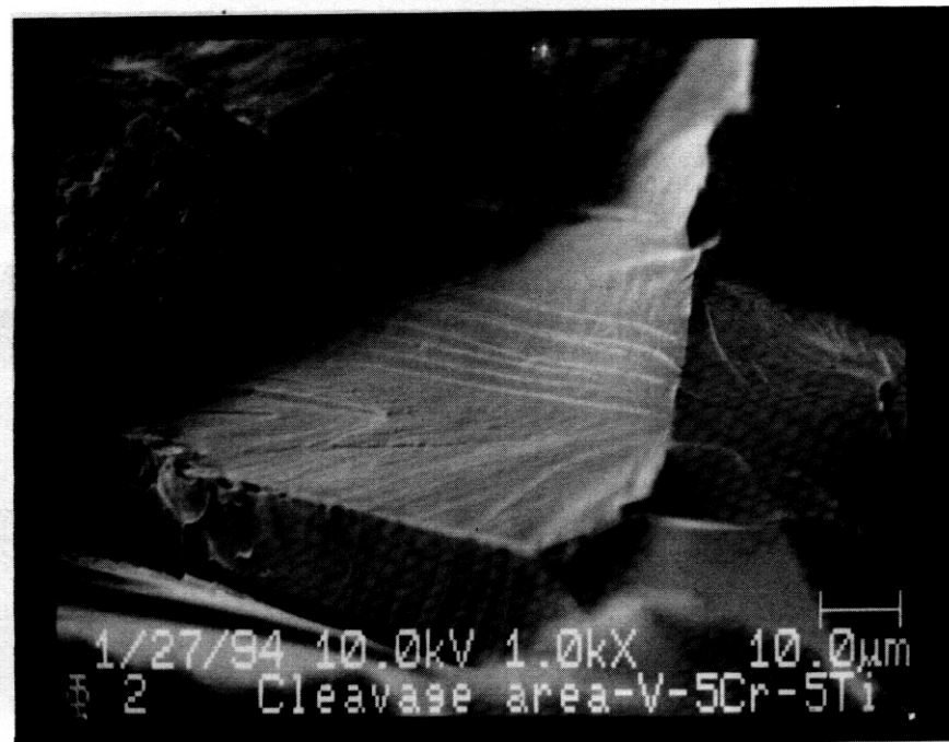
Fig. 8. Cleavage fracture surface used for comparison with grain boundary surfaces. The analysis appears in Table 1.
