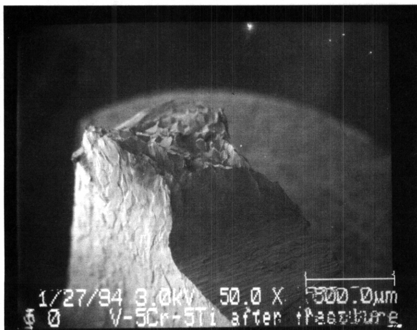
Fig. 1. Macro view of fractured specimen of V-5Cr-5Ti.
