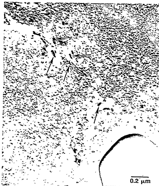
Fig. 5. Matrix and grain boundary precipitates in CuNiBe heat #46546.
