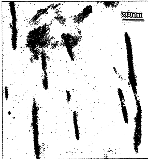
Fig. 4. Micrograph of needle-like carbonitrides in the 7Cr-2WVTa steel.
