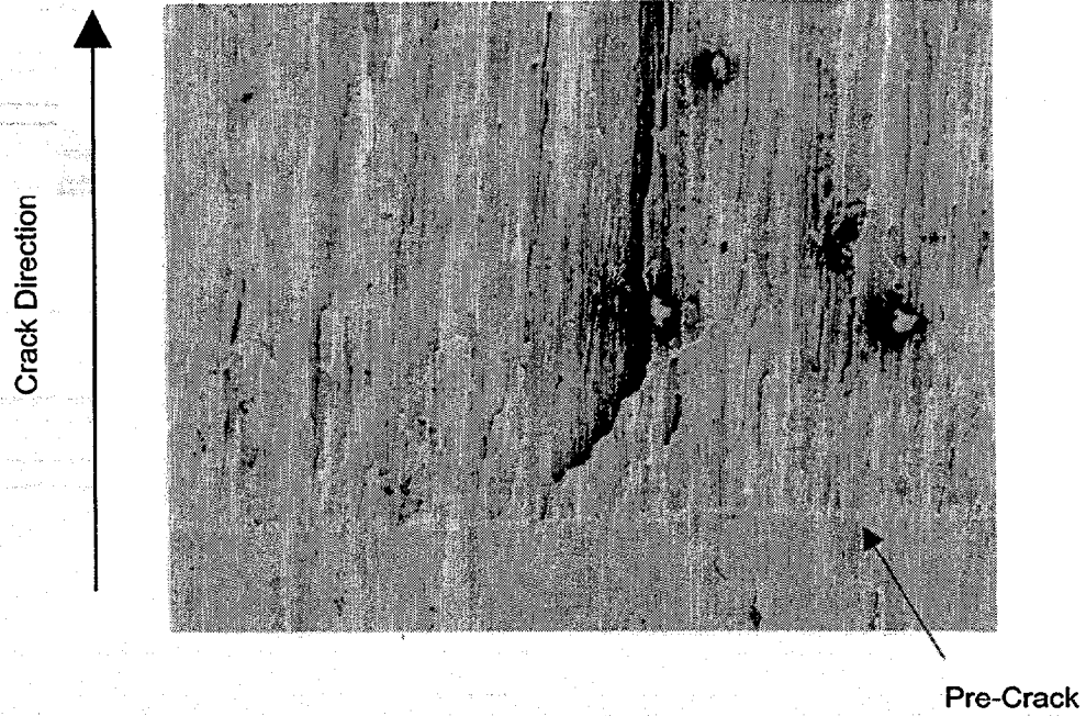
Figure 10. SEM image of fracture surface in C-L orientation tested at 25°C.
