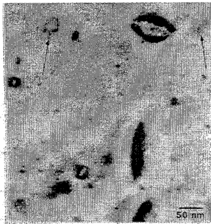
Fig. 6. Cavity formation at dislocation loops in \text{Al}_2\text{O}_3 irradiated with 1 MeV H ions at 650^\circ\text{C} to 1.7 \times 10^{22} H/m 2 . The microstructure corresponds to an irradiation depth of \sim 9 \mu\text{m} (1 \mu\text{m} from the peak implanted region).
