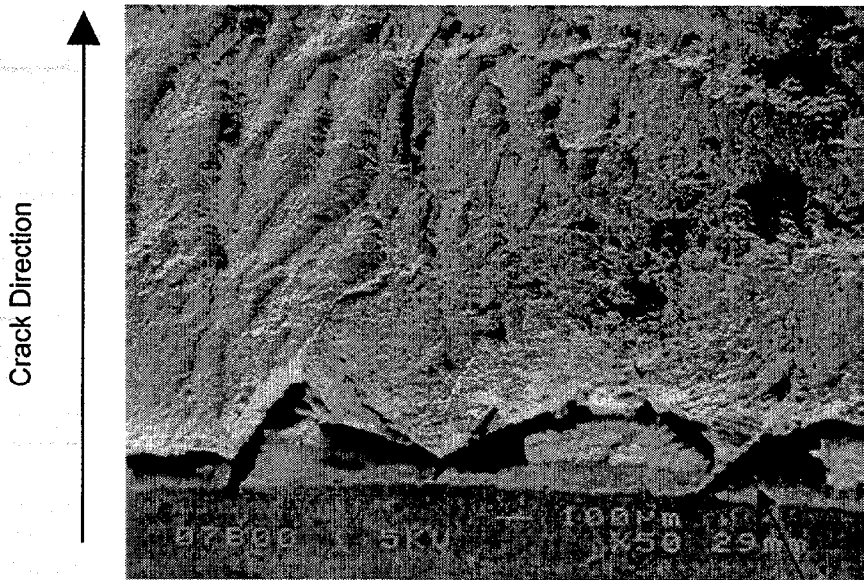
Figure 7. SEM image of fracture surface in L-R orientation tested at -70^{\circ}\text{C} .
