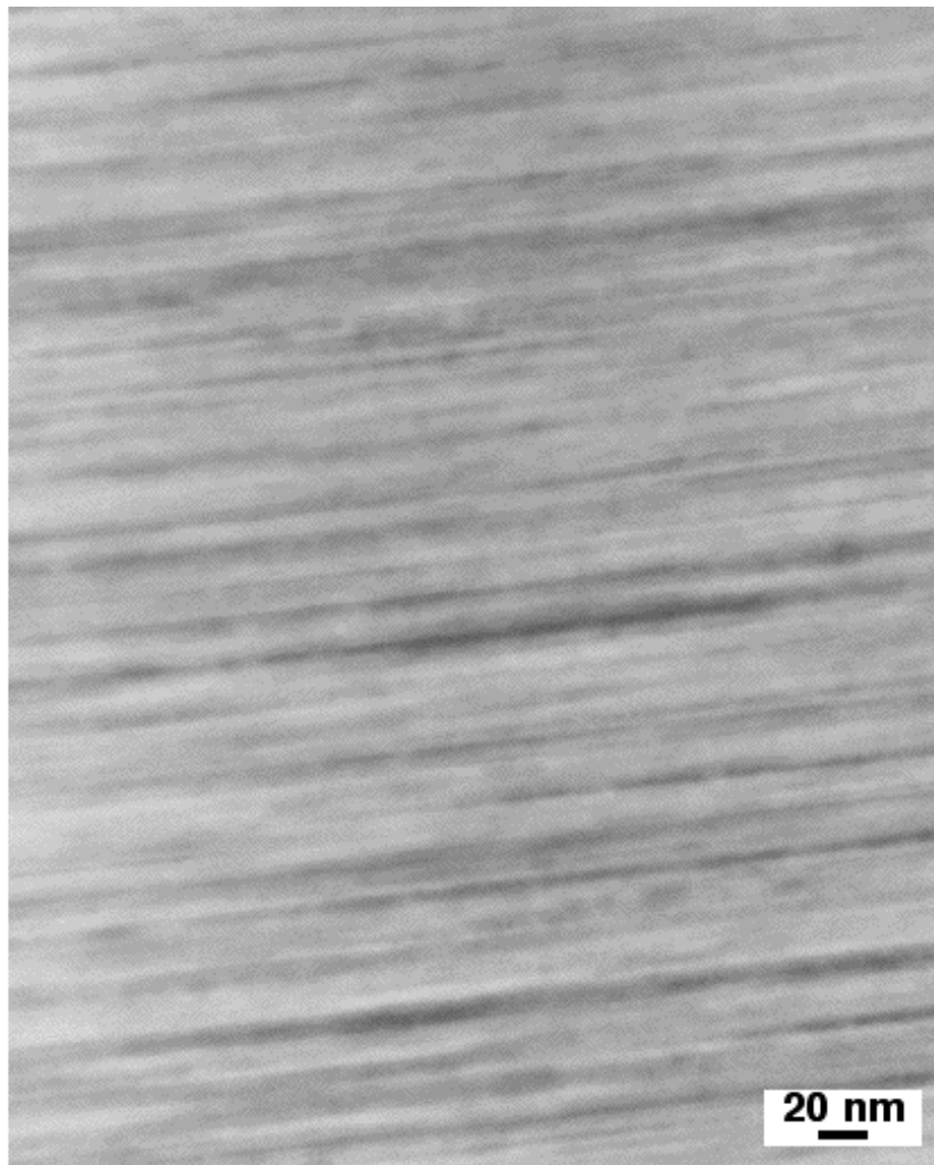
Fig. 3. Microstructure of Si 3 N 4 irradiated with 710 MeV Bi ions.
