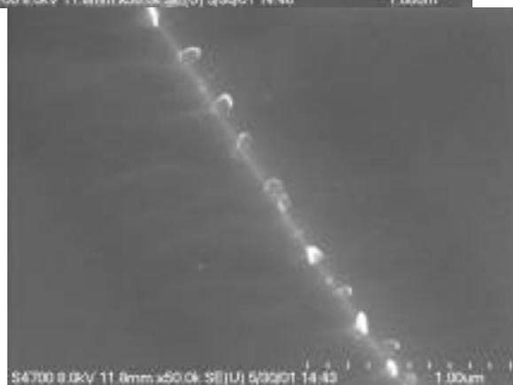
Fig. 7. High-resolution SEM images showing small particles (50-100 nm) at (a) grain boundary A and (b) grain boundary B in Fig. 6.
