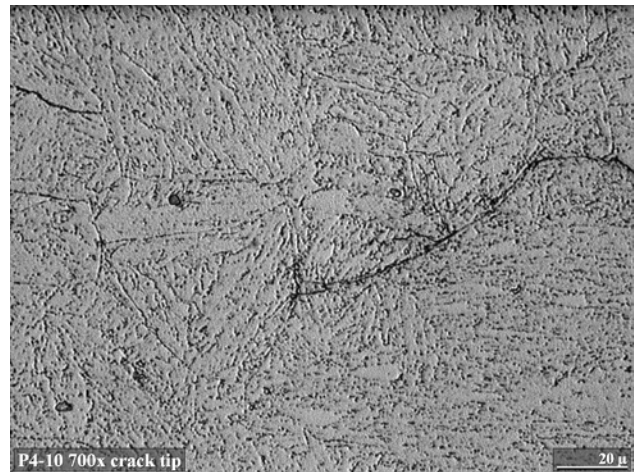
Figure 2. Crack tip of Figure 1 at higher magnification
