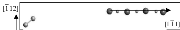
Fig. 3. Atomic plot showing the emission of a self interstitial atom that forms a \langle 111 \rangle crowdion.
