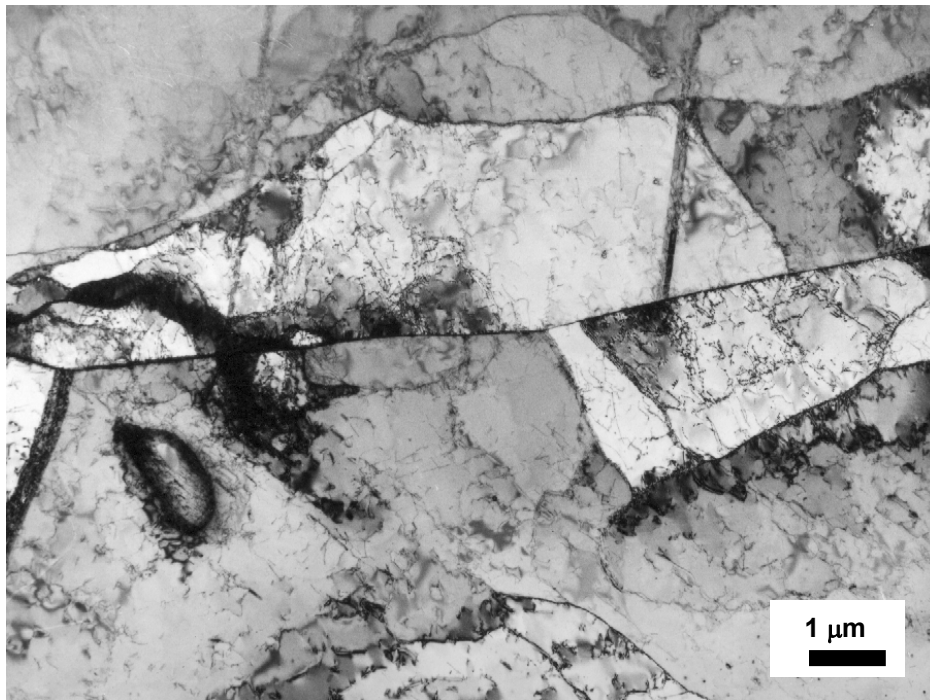
Fig. 1. Microstructure of the unirradiated steel 12X18H9T from the template cut out from the upper flange of the BR-10 reactor first vessel.
