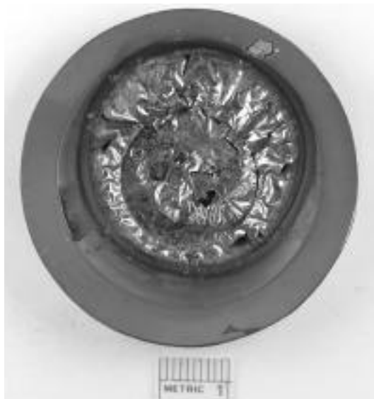
Fig. 3. Photograph of the Er 2 O 3 /V coated specimen after exposure to Li. A pool of liquid Li was in the center of the bowl at up to 500°C.
