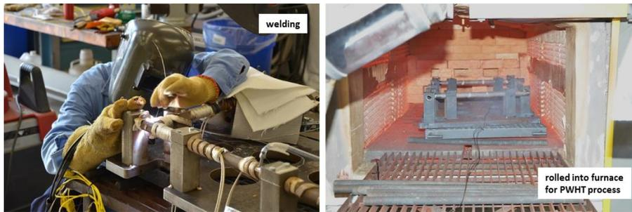
Figure 2. Welding and heat treatment. At left, completion of a saddle weld at the bottom of the loop. At right, the loop is shown within the box furnace for post-weld heat treatment (PWHT).
