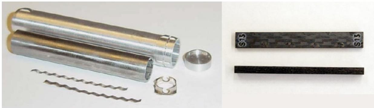
Fig. 2. HFIR rabbit capsules before assembly (left: capsule housing, specimen holder, and springs are shown on top, middle, and bottom, respectively, and capsule end cap and centering thimble are shown on right) and a pair of HNLS composite samples. Length of specimens and specimen holder are about 5 mm.
