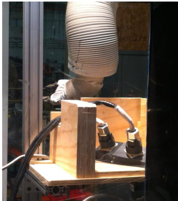
Figure 7. Remote handling mockup for FMITS electrical connections.
