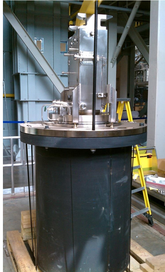
Figure 2. Target seal test tank which will be adapted to test FMITS-type core vessel seal.
