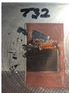
Figure 8. A tungsten foil, 250 µm thick cracked and shattered during a welding test with a copper interlayer and steel baseplate.
