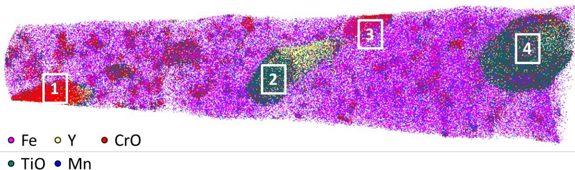
Figure 1. An ion map shows the elemental distribution within this particular needle. Four large particles are highlighted for subsequent examination. Analysis revealed a grain boundary close to particles #2 and #3. The grain boundary only shows slight enrichment in C, but no major segregation of other alloying elements. The bulk composition of each overall particle is listed in Table 2, but a more complete analysis revealed particle #4 exhibited a Ti(Cr)N core with a Ti(Cr)O shell.
