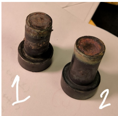
Figure 1. Two tungsten alloy thimbles that were tested under high heat flux conditions with He cooling at Georgia Tech #1) WL10 alloy #2) MT-185 alloys.
