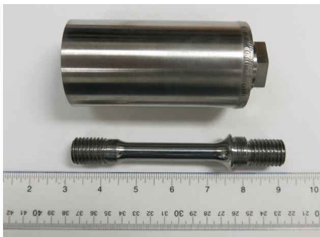
Figure 1. Images of (bottom) Hollow tensile specimens (top) 316L catch cup for lithium.
