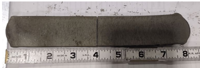
(f) 14 th pass 77.8% reduction pre anneal sectioned
