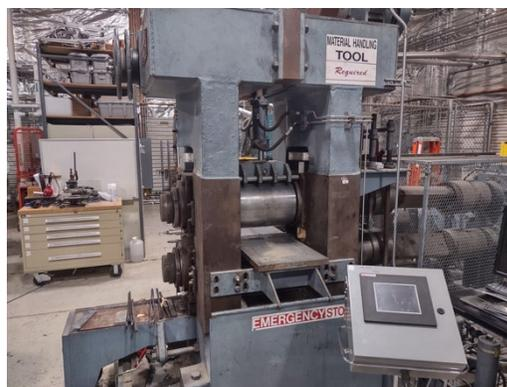
**Figure 4.** Preheating Lucifer Furnace and Waterbury Farrell Rolling Mill.
