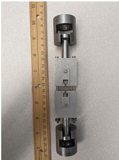
**Figure 2.** Shoulder-loaded TZM tensile fixture.
