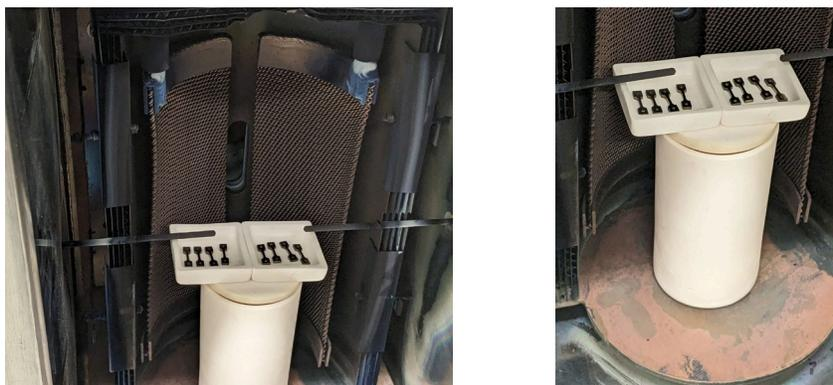
**Figure 9.** Tensile samples were annealed at 1300°C (under 5-10 mTorr vacuum) for different durations (6 h, 12 h and 24 h).
