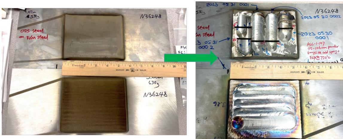
**Figure 2.** Two large-area ODS steel deposits (#1 and #2) were cold sprayed onto P92 substrates, respectively. The #1 plate was used for optimization of the FSP step. The #2 plate was FSP processed with an 8-pass raster.
