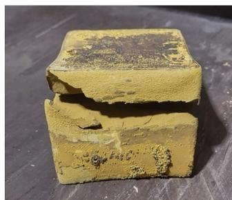
(c) After 6<sup>th</sup> pass; Left: pre anneal (rotated 90° before taking a photo); Right: Post anneal
