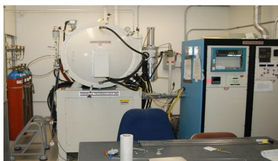
**Figure 5.** Left: CM Furnace utilized for 1200°C annealing during hot rolling process. Right: Thermal Technologies/Brew Furnace for degassing hydrogen.
