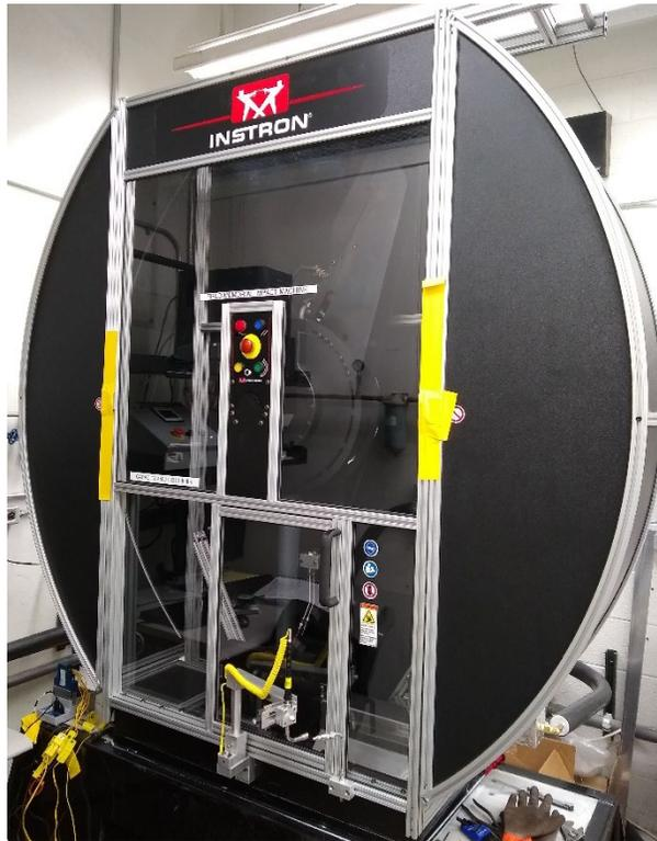
**Figure 2.** Instron Charpy impact frame equipped with an MPM in-situ heating/cooling stage.
