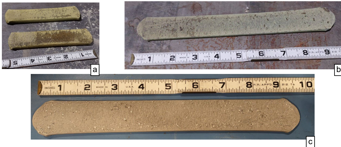
Figure 4. Hot rolled plates obtained from sintered 90 wt.% W–Fe–Ni alloy (a) 66R thickness reduction (before final annealing): 2023/1-in/01 & 02 (b) 83R thickness reduction (before final annealing) (c) 83R thickness reduction (after final annealing): 2023/1-in/03.
