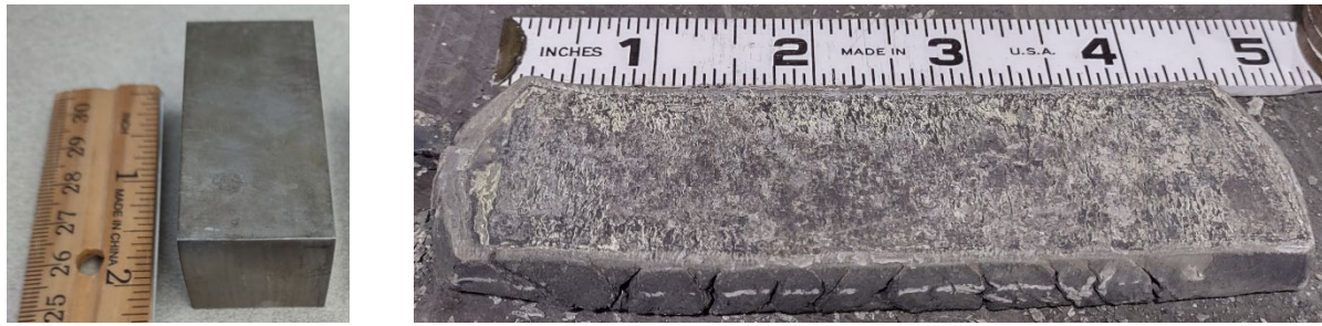
Figure 13. Hot rolled 90W–Fe–Ni (#2023/1-in/04); (a) before; (b) after 6 th pass (66R) before annealing.
