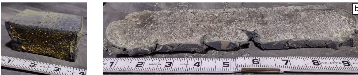
Figure 9. Hot rolled 90W–Fe–Ni plate (#2023/2-in/03); (a) after 4 th pass (18R) before annealing; (b) after 12 th pass (83R) after annealing.
