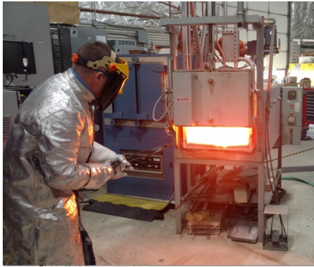
Figure 1. Preheating Lucifer Furnace and Waterbury Farrell Rolling Mill.
