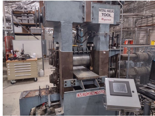
Figure 1. Preheating Lucifer Furnace and Waterbury Farrell Rolling Mill.
