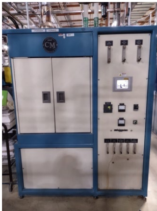
Figure 2. Left: CM Furnace utilized for 1200°C annealing during hot rolling process; Right: Thermal Technologies/Brew Furnace for degassing hydrogen.
