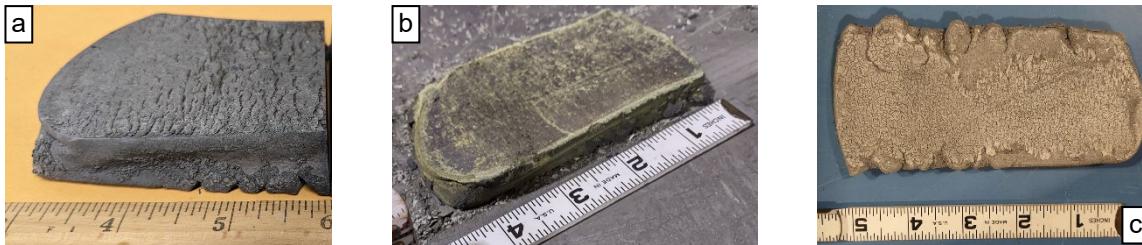
Figure 7. Hot rolled 90W–Fe–Ni plate (#2023/2-in/02B); (a) used one half of the 67R plate (see Figure 6c) for additional hot rolling; (b) after 24 th pass (79R) before annealing; (c) after 26 th pass (83R) after annealing.
