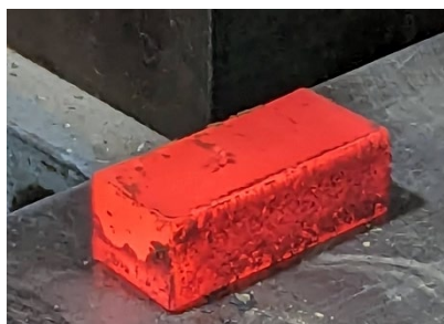
(a) Before hot rolling (1" thick x 1" wide x 2.25" long pieces) and during hot rolling
