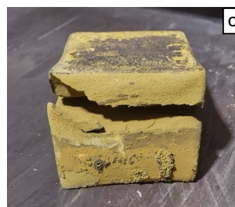
Figure 5. Hot rolled 90W–Fe–Ni (#2023/2-in/01); (a) before hot rolling; (b) sample got split horizontally during the 6 th pass - before annealing (c) after annealing.
