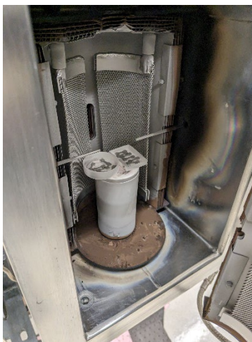
Figure 16. Tensile samples annealed at 1300°C for 24 hours using the MRF furnace.
