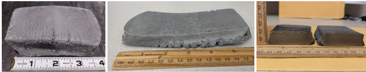
Figure 6. Hot rolled and annealed 90W–Fe–Ni plate (#2023/2-in/02A); (a) after 12 th pass (44R); (b) after 20 th pass (67R); (c) plate (67R) was sectioned in two pieces, one piece was rolled further, see Figure 7.
