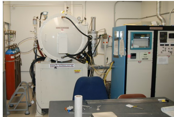
Figure 2. Left: CM Furnace utilized for 1200°C annealing during hot rolling process; Right: Thermal Technologies/Brew Furnace for degassing hydrogen.
